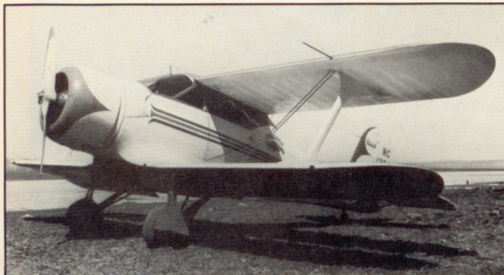
The third Model 17 and, first production Beechcraft, Model B17L, was the baby of the Staggerwing line with the 225-hp Jacobs engine.
